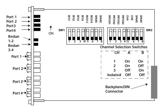
Figure 3-1. 10BASE-FL Module Dip Switch Locations
